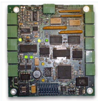
Local Alarm Module 16 Water detects 2 grounds fault
